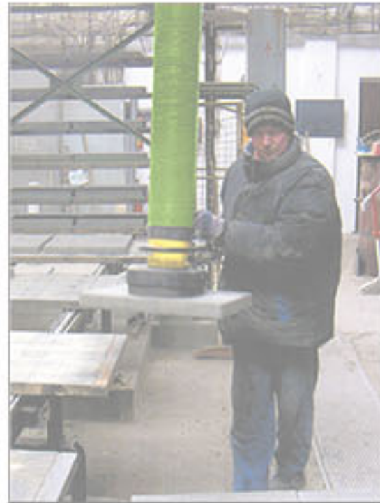
▲ 塑板搬運作業 Plastic Plank / brick
