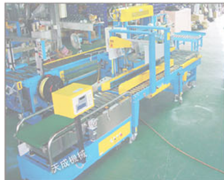
封箱磅重作業輸送機 Carton Sealing + Strapping + Weighting Conveyor System
