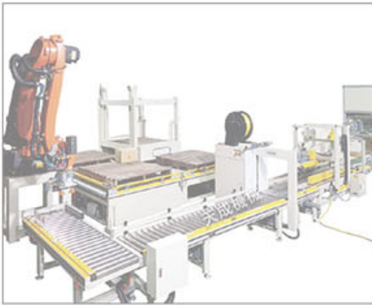
全自動包裝堆棧系統 Fully Auto Palletizing with Robot
